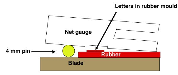
• If the ruler touches the rubber, but not the pin, the rubber is too thick, so the extra gap between the ruler and the pin shall be measure with a thickness gauge. The maximum thickness which may be introduced between the pin and the ruler (without pushing up the ruler) shall determine the value of the extra thickness of the rubber.
