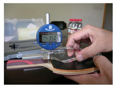
The diameter of the pin touching the blade shall be between Ø4.5 and Ø5.0 mm.
